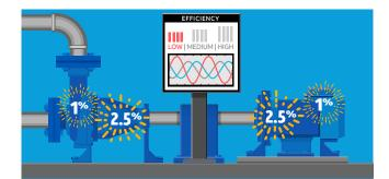
For a 100 hp motor operating 8,000 hours per year, a correction of the voltage unbalance from **2.5**% to **1**% will result in electricity savings of **9,500** kWh.<sup>13</sup>
